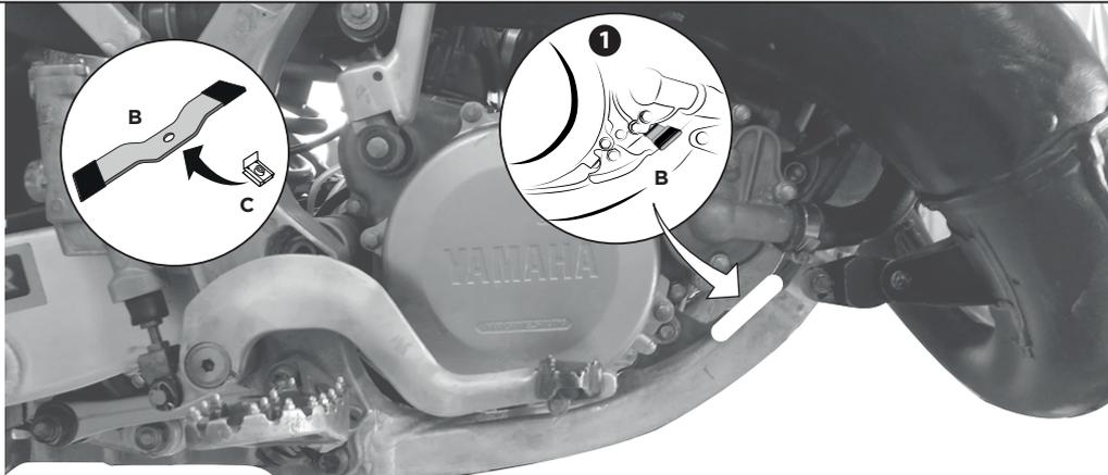
**Attach the threaded Clip (C) to the Bracket (B) and then position the bracket behind the frame as indicated in the image.**
