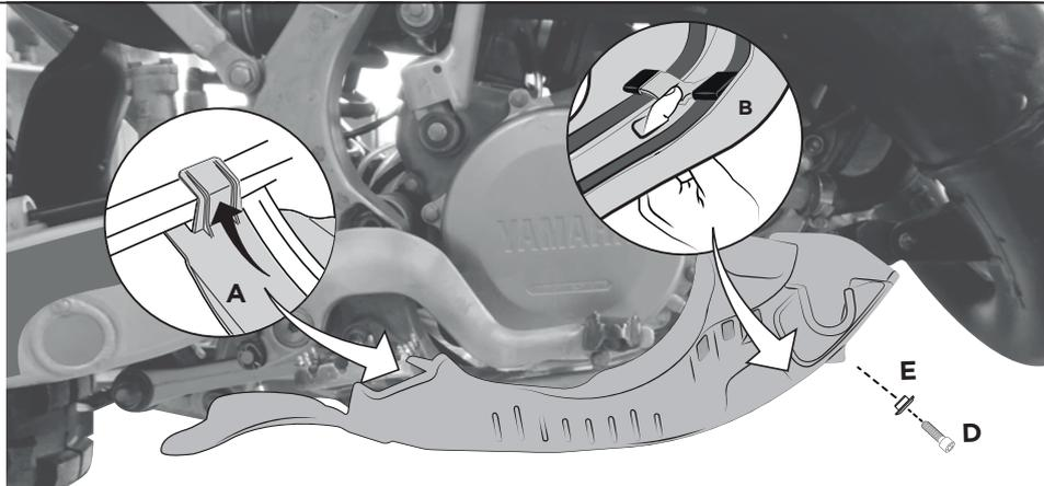
**Hook the back of the skid plate over the frame as indicated in the image and push the skid plate firmly against the frame. Using the index finger, reach through the skid plate and position the bracket (B) as indicated in the image. Insert the bushing (E) and bolt (D) and tighten firmly.**
